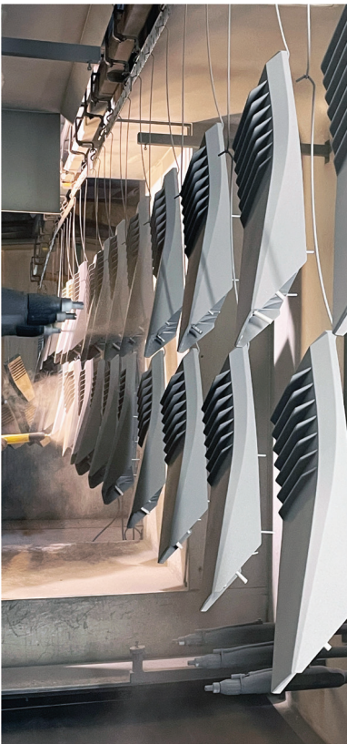
Automatic powder coating arms provide uniform 120 micron thick paint application.
